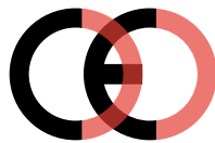
False CE Mark (too close)
